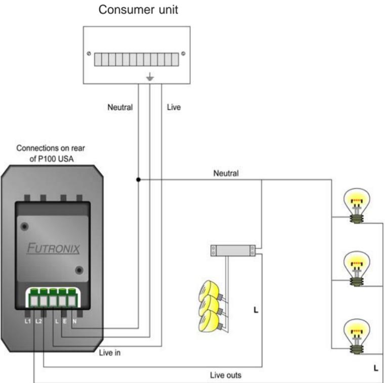
A Typical Wiring diagram for the P100 USA
