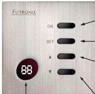
This window is a combined display and Infra-red receiver. The display in normal mode shows the scene selected. In program mode it shows the relevant programming information.
