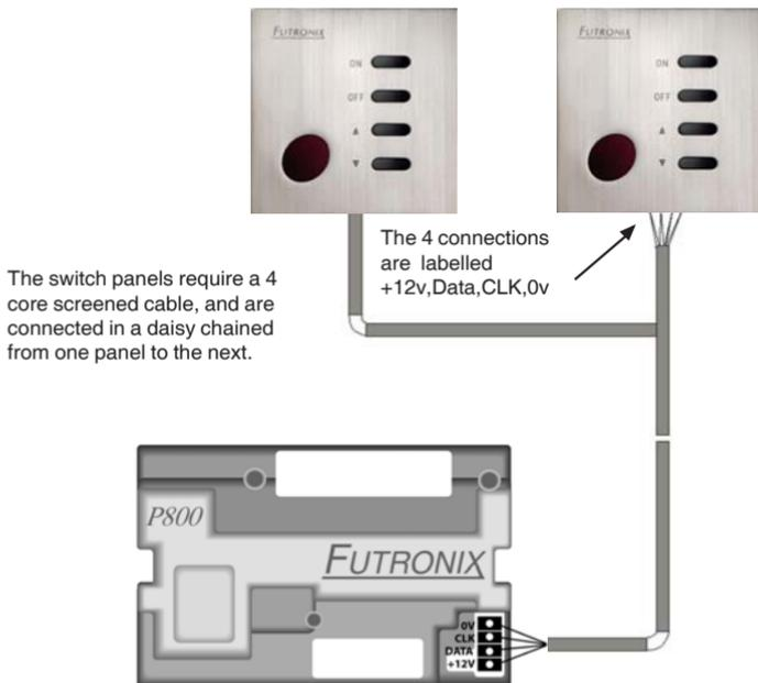
Connect up the cable in accordance with the diagram above. The cores are labelled as follows: [0v, CLK, DATA, 12v]. There can be several switch panels connected to each controller system and cable distances can be up to 150m between switch panels and controllers. The switch panels should be daisy chained together one on to the next etc.
