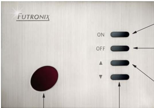
This window is a combined display and Infra-red receiver. The display in normal mode shows the scene selected. In program mode it shows the relevant programming information.
